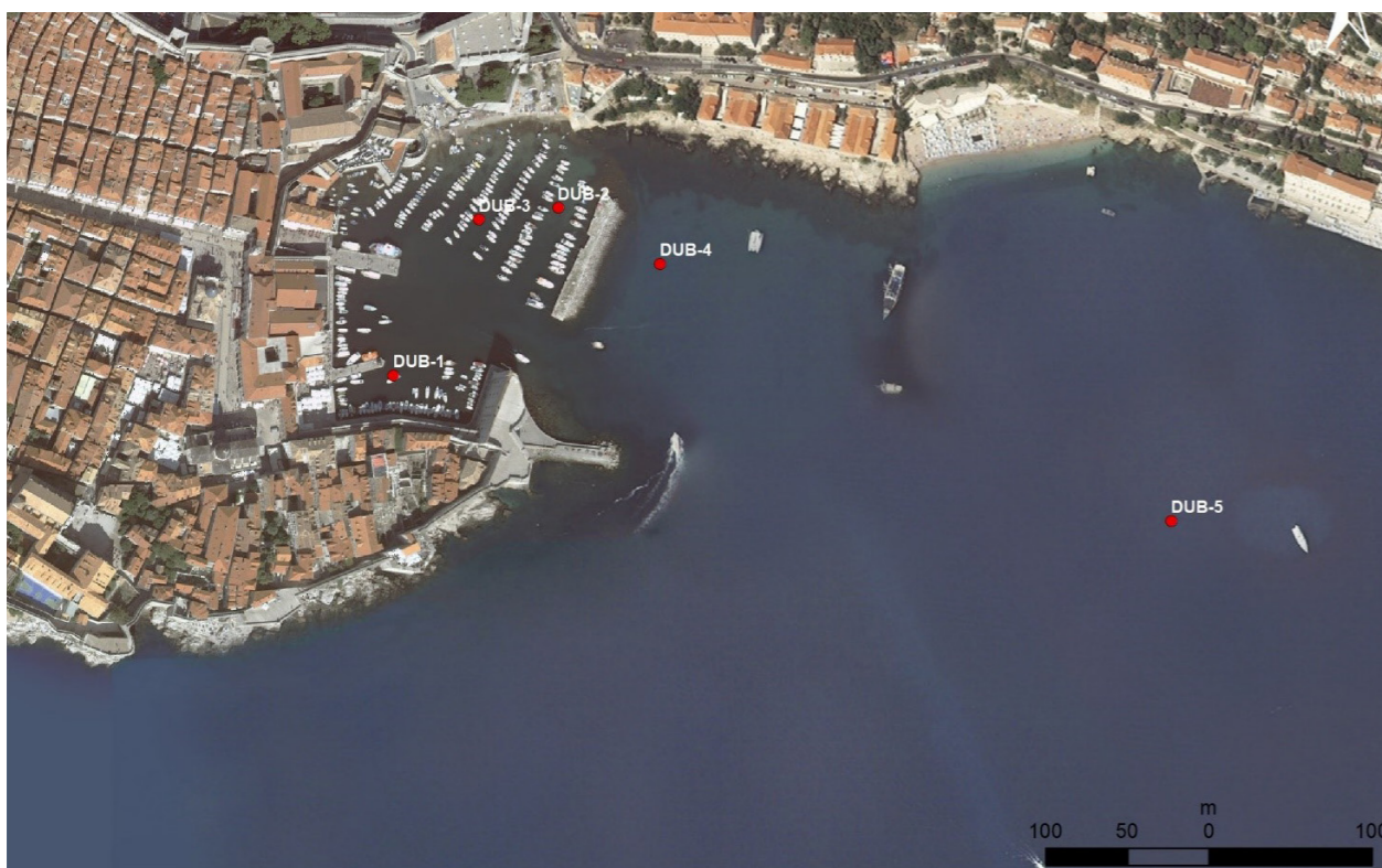
Fig. 24 Positions of geological cores (Croatian Geological Survey)
