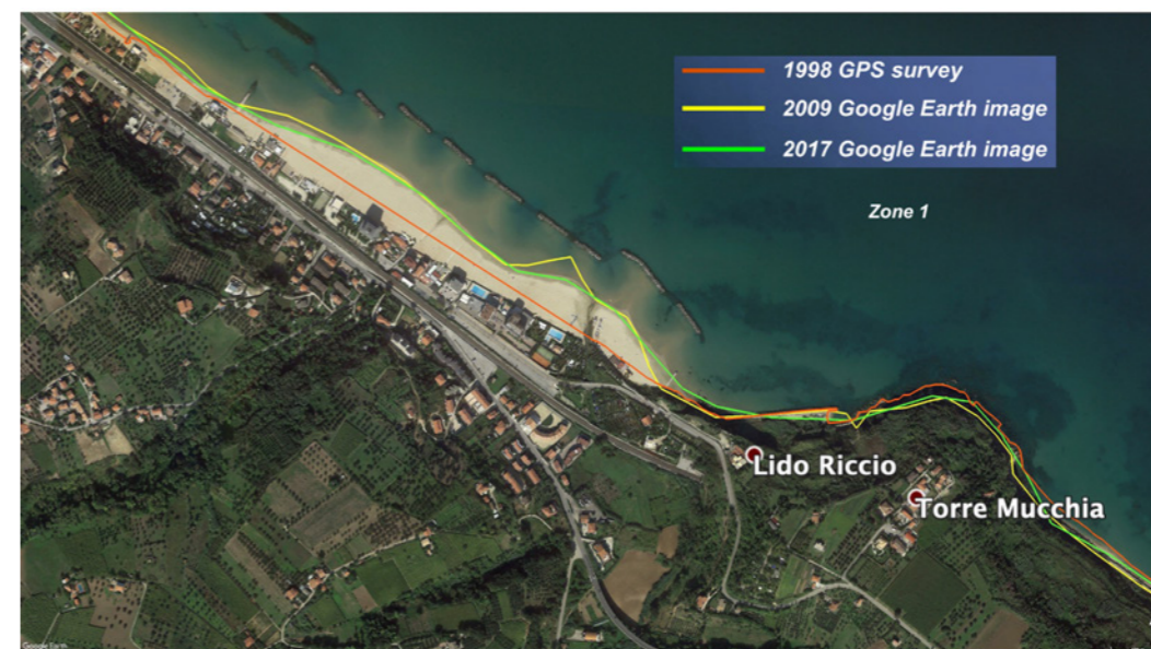
Figure 14. Comparison of the coastline variation from 1998 to 2017 in two sites of Zone1 (refer to Figure 13).
